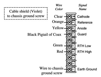
Some cables have connectors on the leads. Cut off the connectors, skin and tin the leads and then wire to the screw terminals on the boards
